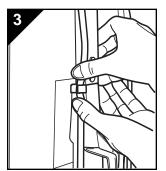
Attach cord to cord clip by pressing cord above and below clip ensuring the cord is fully rested in clip.
